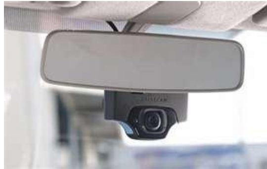
Figure 1. DriveCam Event-Triggered Video Data Recorder
