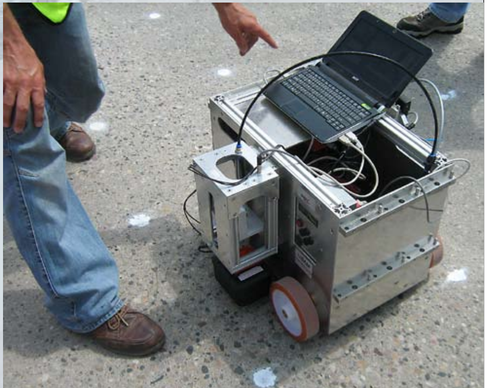
Impact echo device is mounted on a remote-controlled robot in action
