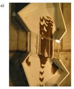
**Figure 11** Sediment deposition pattern at 15 degree skewed culvert model after three-hour operation: a) no design in the expansion, and b) fillet-based design in the expansion
