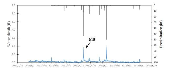
Figure 17 Stage and precipitation records at the culvert site (2012/03/01 ~ 2012/05/31)
