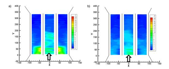
**Figure 7** Mapping of the sediment deposits formed in three culvert boxes after 6-hours: a) without the design placed in expansion; b) with design placed in expansion
