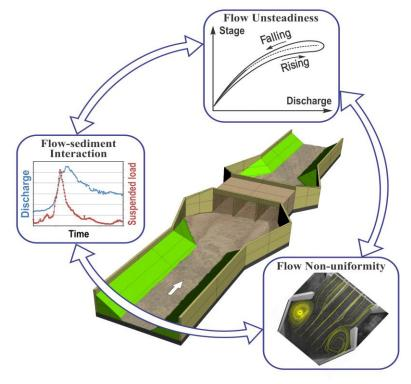
Figure 3 Complexity factors at flow through culverts
