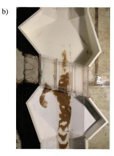
**Figure 10** Sediment deposition pattern at 15 degree skewed culvert model after one-hour operation: a) no design in the expansion, and b) fillet-based design in the expansion
