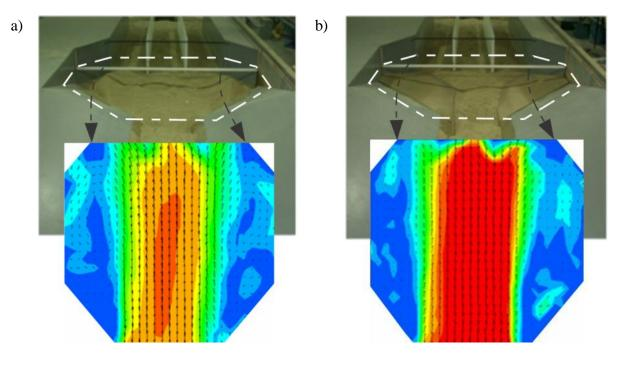
**Figure 9** Velocity distributions upstream the 1:5 culvert model: a) original configuration, b) hydro-cleaning design implemented
