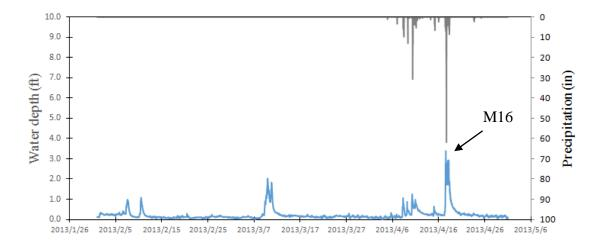
Figure 18 Stage and precipitation records at the culvert site  $(2013/02/01 \sim 2013/4/30)$
