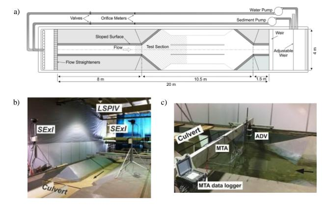
Figure 6 Arrangement of the acoustic sensors for the measurement of sediment deposition in the 1:5 scale culvert model
