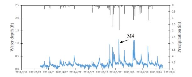
Figure 16 Stage and precipitation records at the culvert site  $(2011/04/01 \sim 2011/06/30)$
