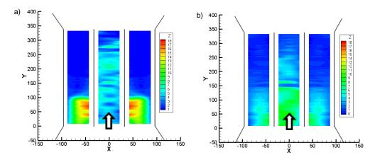
**Figure 8** Mapping of the sediment deposits formed in three culvert boxes after 12-hours: a) without the design placed in expansion; b) with the design placed in expansion
