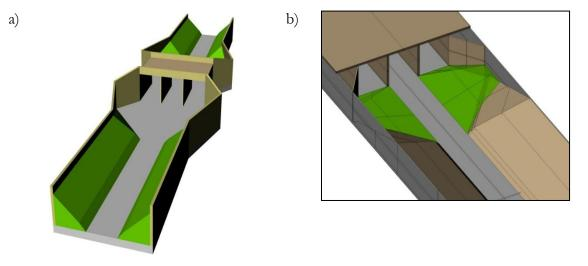
Figure 4 Schematic of the TRGB-G1-01 culvert tested in the study: a) original configuration:b) self-cleaning design established through TR 545
