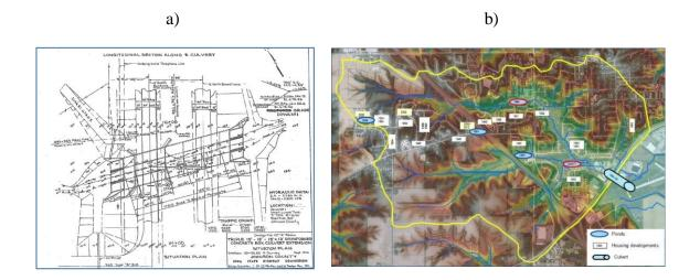
**Figure 12** a) Construction drawings for the culvert for monitoring; b) drainage area for the culvert
