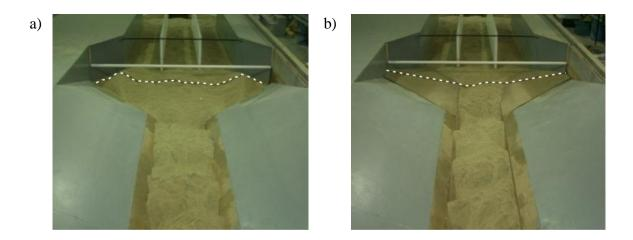
**Figure 5** Sediment deposition patterns without and with fillet-based self-cleaning system: a) no hydro-cleaning design, b) hydro-cleaning design constructed
