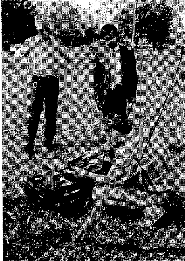
Figure 6.6. Base station GPS data collection
