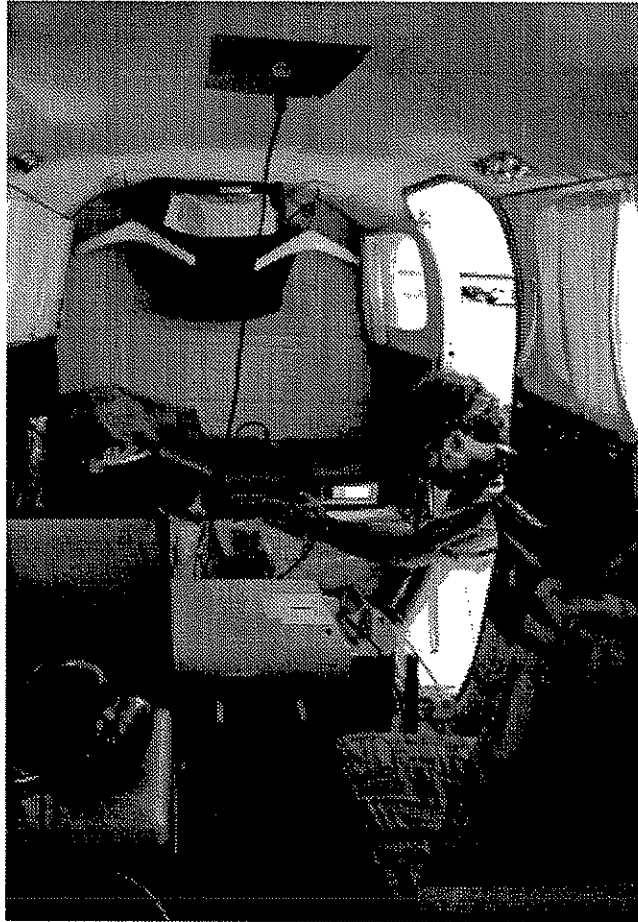
Figure 3.3. Camera and receiver inside aircraft.
