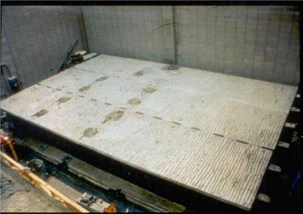
Figure 2.1. Photograph of laboratory PCDT unit bridge [4].
