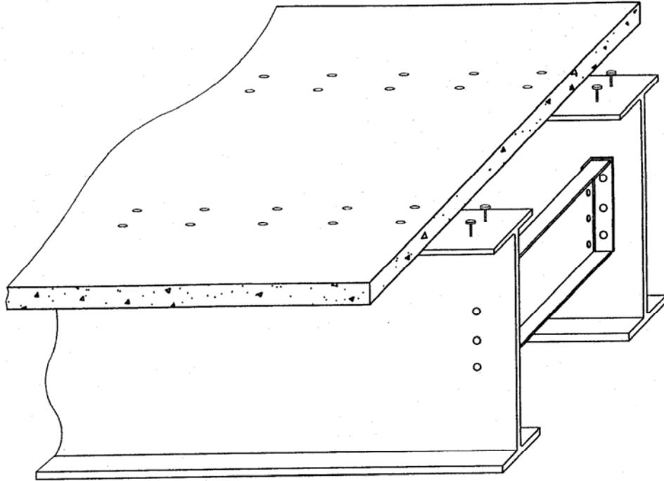
Figure B.1. Black Hawk County modification of the ends of the PCDT units.
