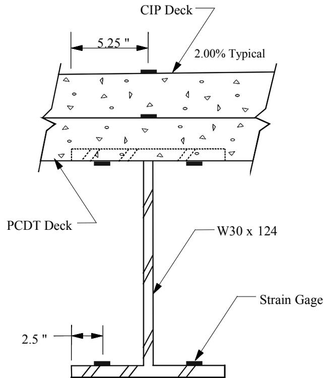
Figure 4.1. Typical location of strain gages.
