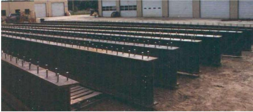
Figure 3.8. Photograph of shear studs used in PCDT units.
