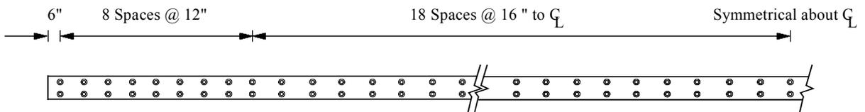
Figure 3.7. Location of shear studs for PCDT units, single beam shown.
