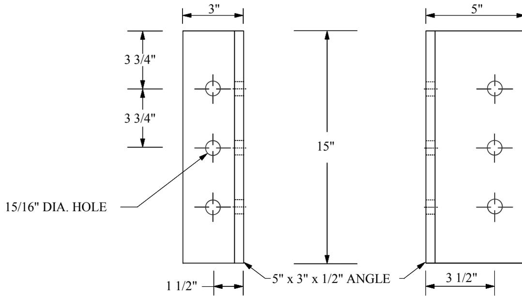
Figure 3.4. Details of diaphragm angles.
