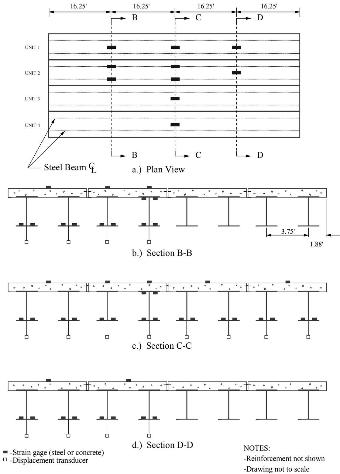
Figure 4.4. Location of strain gages used in first service load test.
