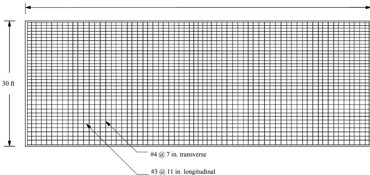
Figure 3.21. Reinforcement details for CIP deck.
