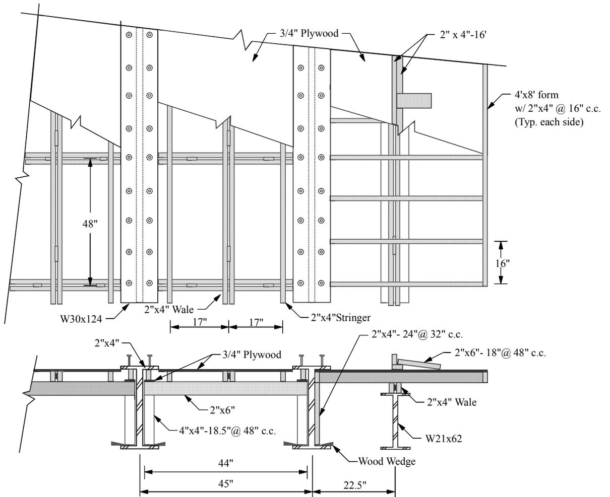
Figure 3.10. Formwork used to cast PCDT units.
