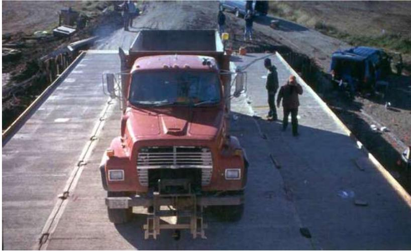
Fig. 4.8. First service load test, truck in position C3.
