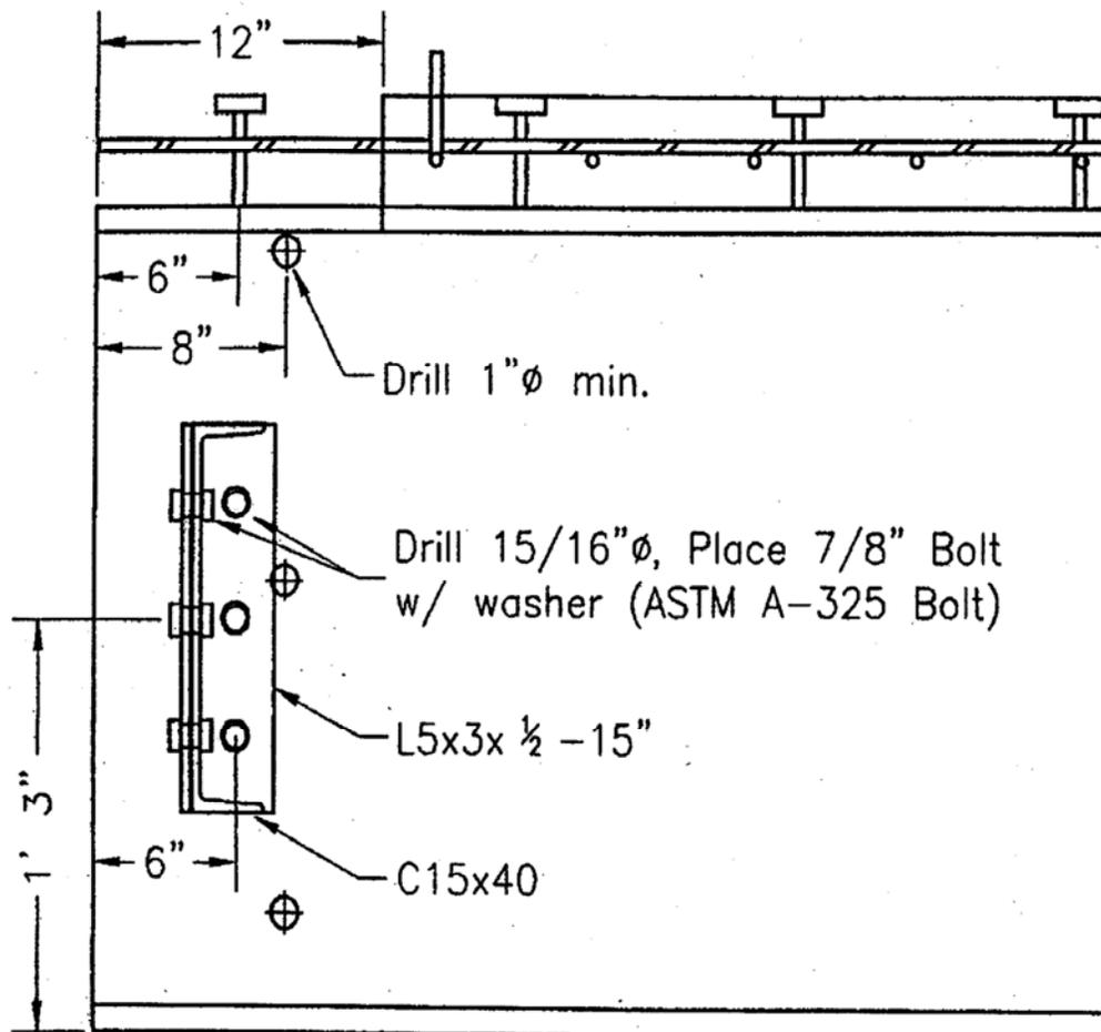
Figure B.3. Steel beam profile showing location of continuous transverse reinforcement.
