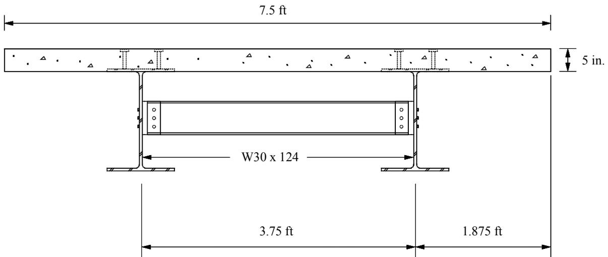
Figure 3.1. Cross section dimensions of PCDT units used in field demonstration bridge.
