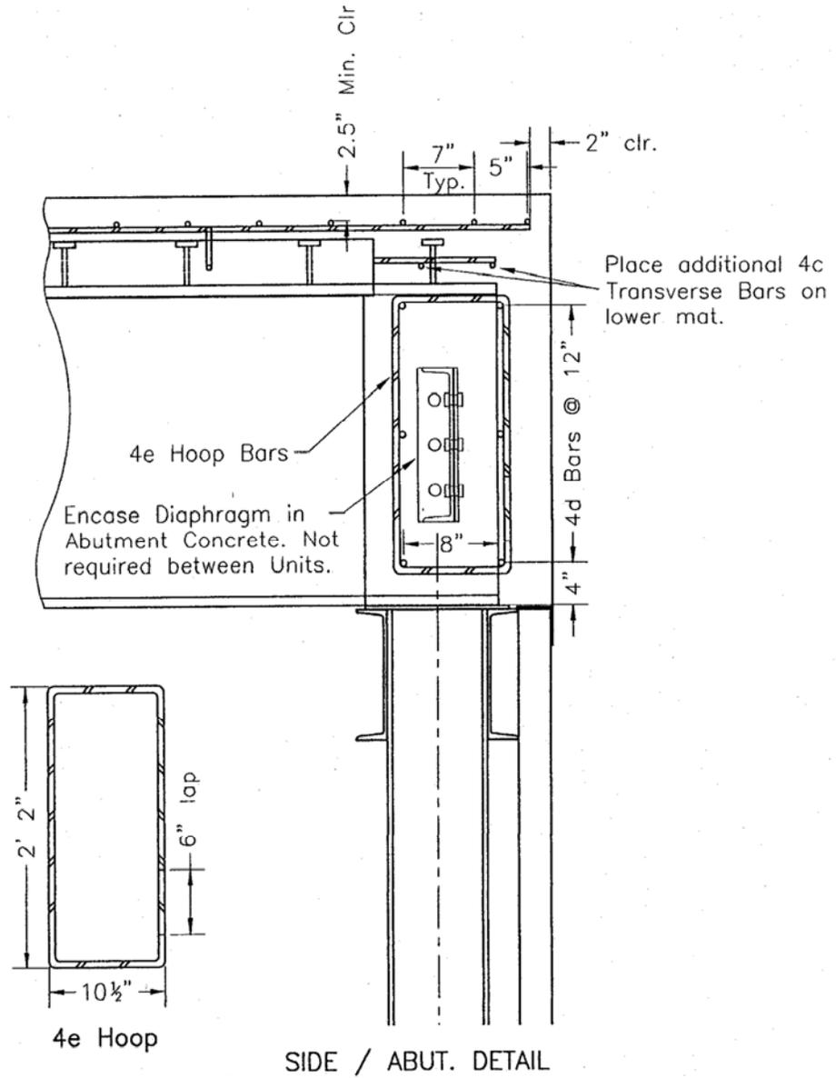
Figure B.2. Reinforcement details for concrete end diaphragms.
