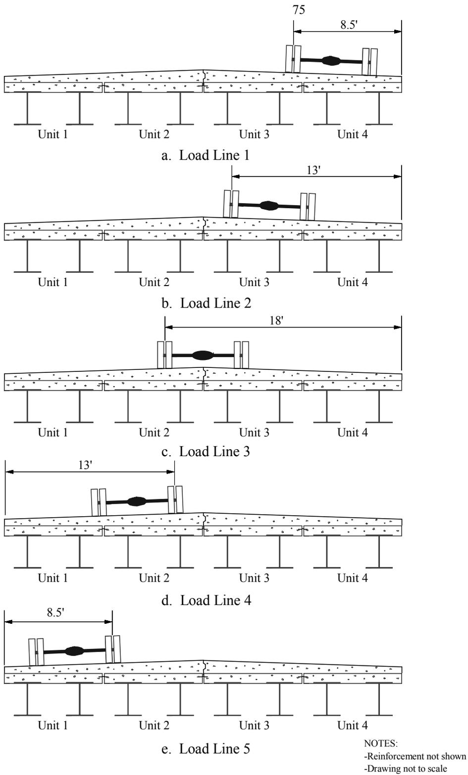
Figure 5.6. Truck load line locations, second and third service load test, Truck No. 23.
