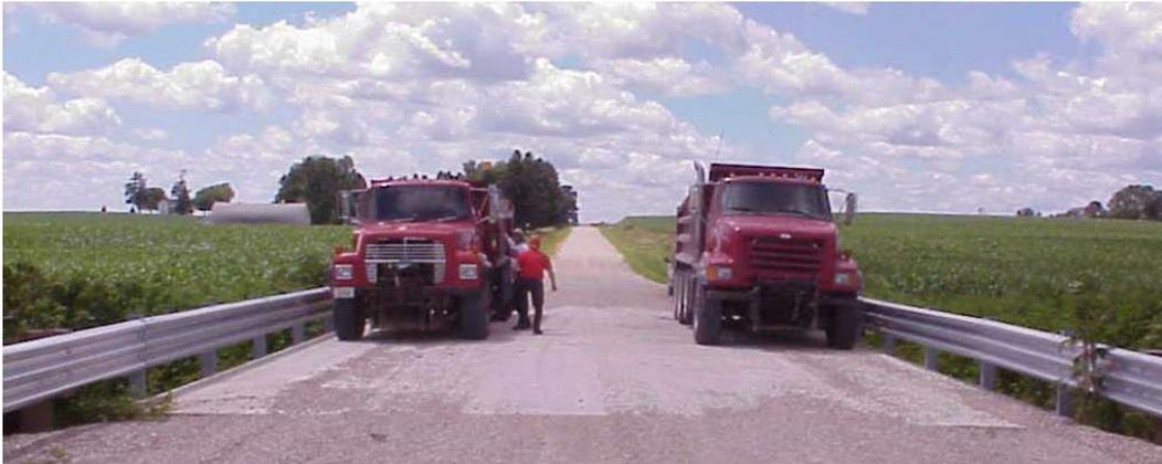
b. End view of replacement bridge during service load testing
