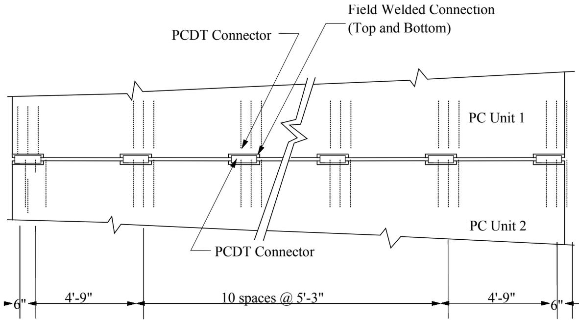
Figure 3.3. PCDT connector-plan view.
