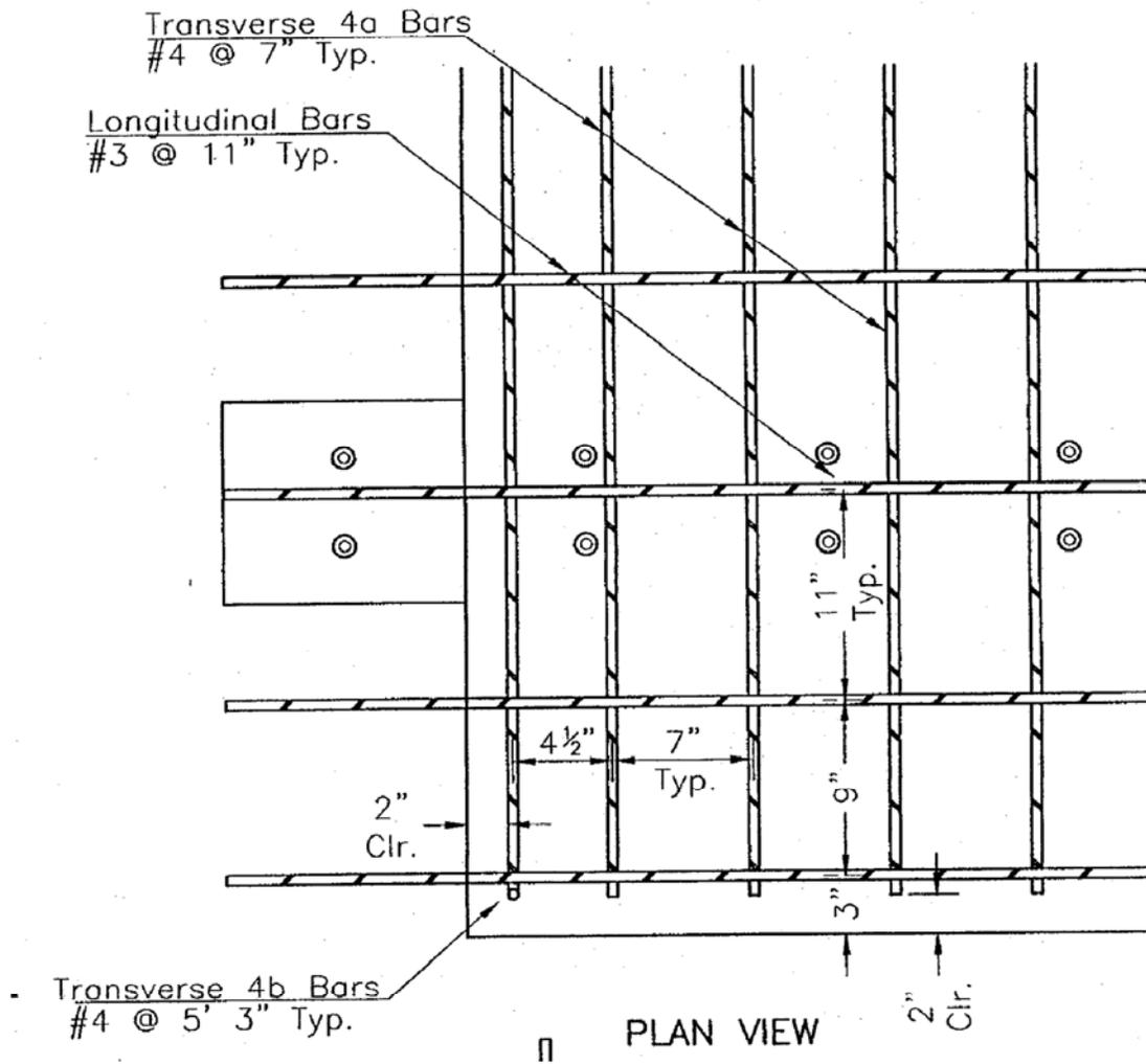
Figure B.4. Black Hawk County modified reinforcement spacing at PCDT ends.
