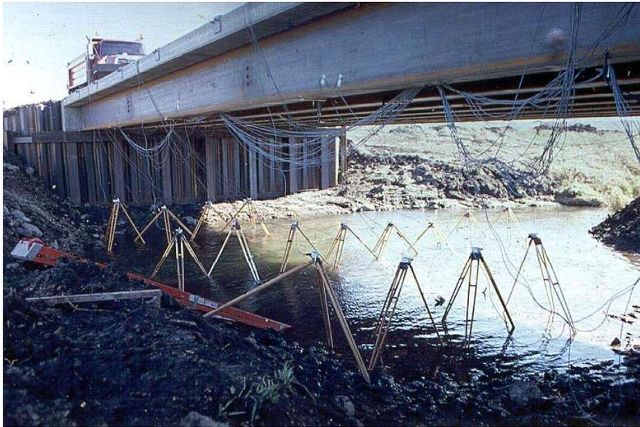
Figure 4.5. Photograph of displacement transducers on tripods during service load tests.
