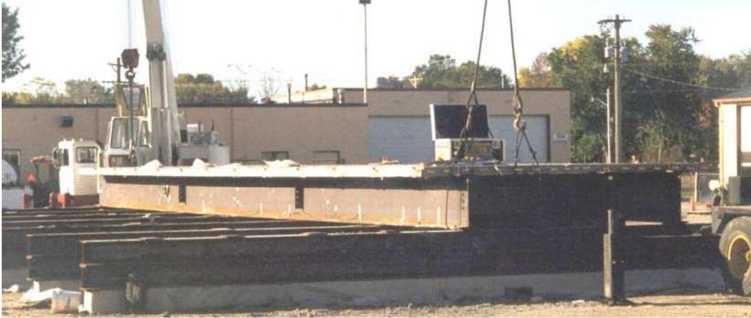
Figure 4.3. Data acquisition cargo box secured onto PCDT Unit 2.
