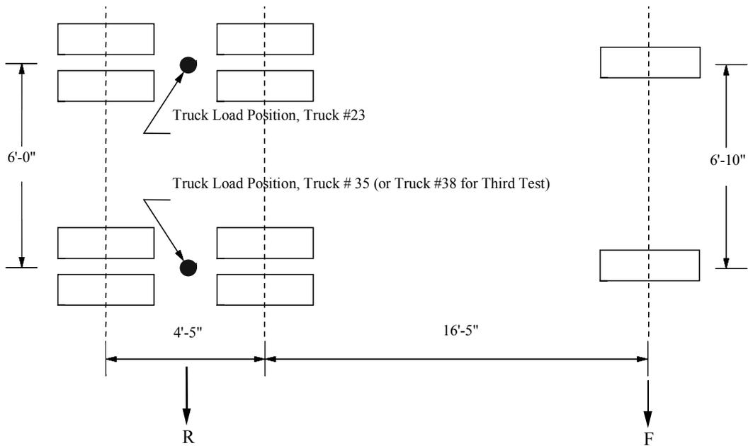
Figure 4.10. Plan view of live load used for second and third service load test.
