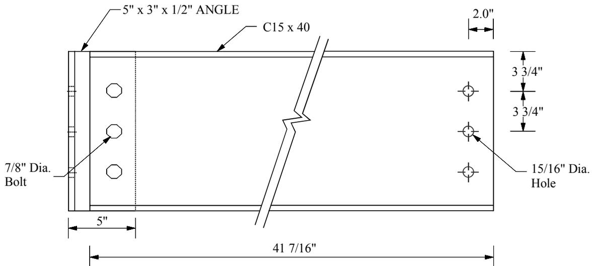
Figure 3.5. Details of diaphragm channels.
