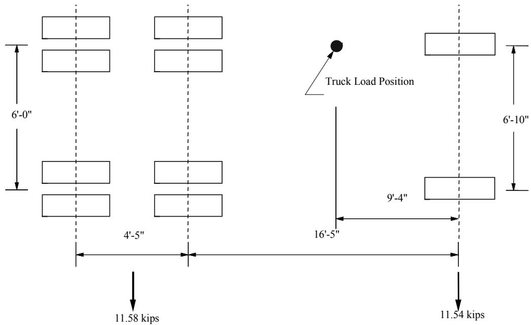
Fig. 4.6. Plan view of live load used for first service load test: Truck No. 23.
