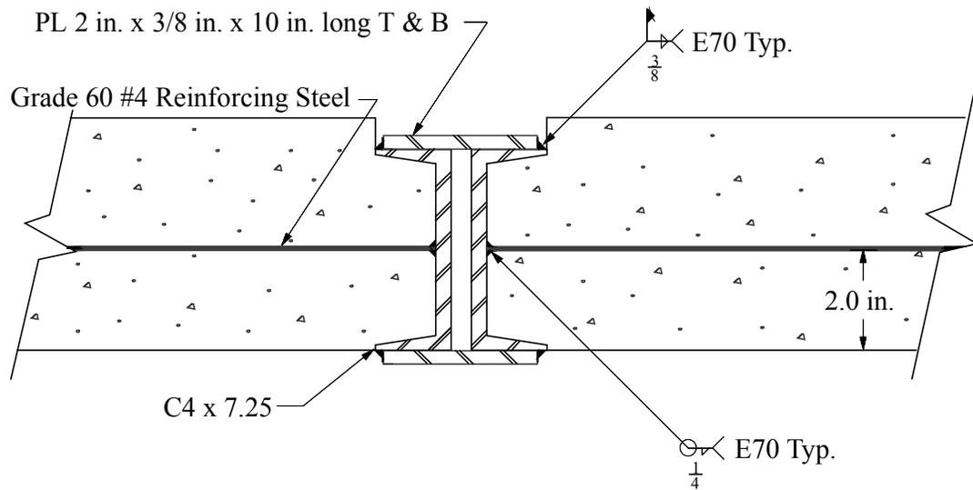
Figure 3.18. Side view of PCDT connection after adjacent units are welded together.
