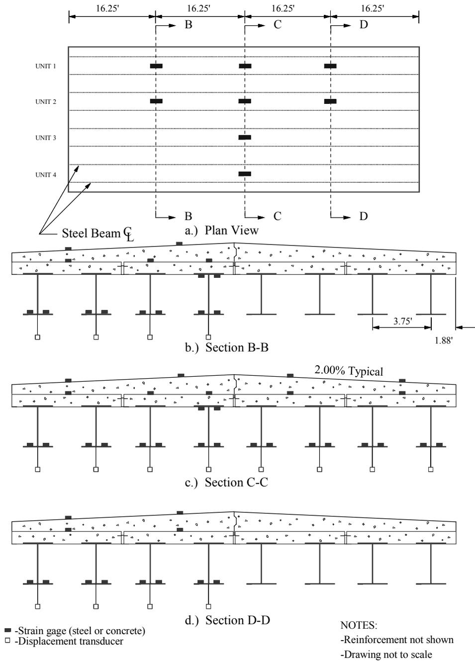
Figure 4.9. Location of strain gages used in second and third service load test.
