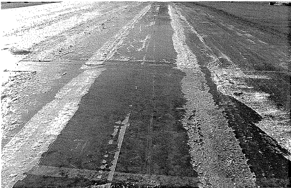
Figure 43. Ice sheet after test number 14 with blade 2, high download, 30^\circ blade angle.
