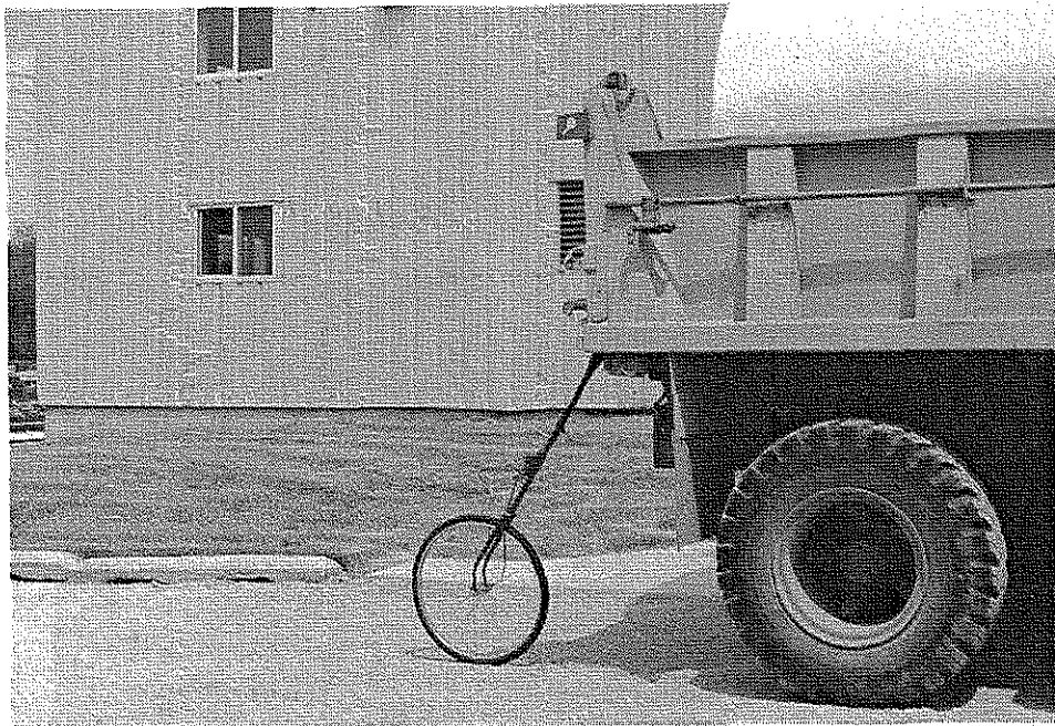
Figure 9. Fifth wheel used to record truck's speed during tests.
