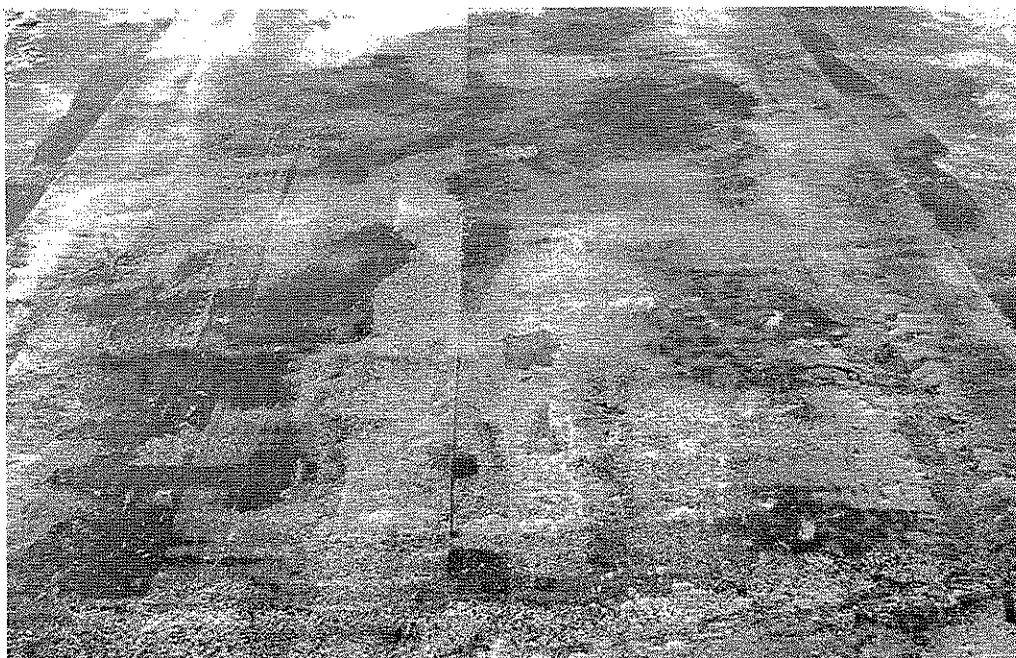
Figure 45. Ice sheet after test number 22 with blade 3, low download, 30^\circ blade angle.
