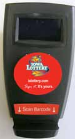
Ticket self-checkers can check both lotto and instant-scratch tickets.
