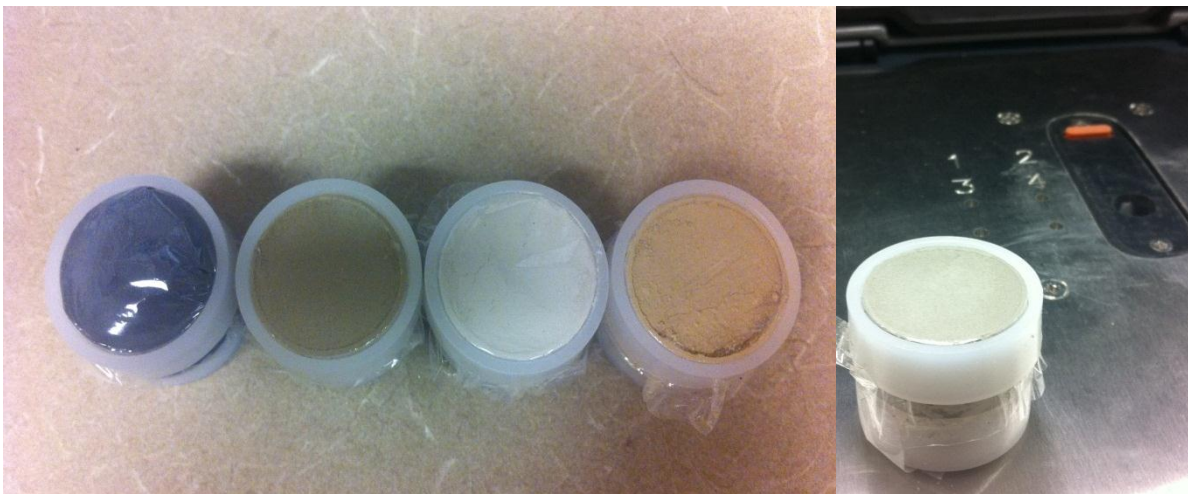
Figure 2. Cementitious materials in sample holders
