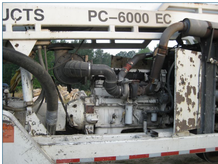
Figure 64. 500 HP, 15 liter engine used to power grinding head
