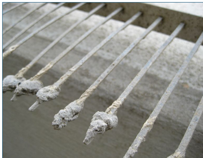
Figure 22. Excessive buildup of hardened mortar on tines
