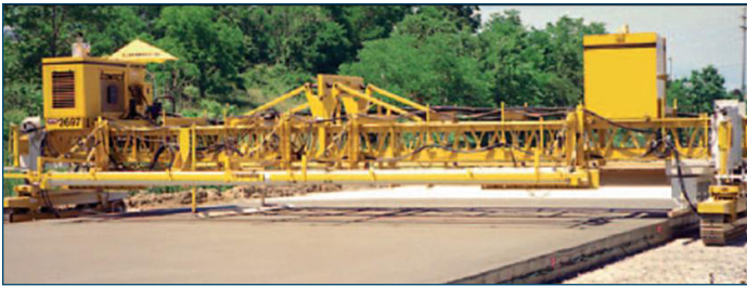
Figure 49. Texture-cure machine manufactured by GOMACO
