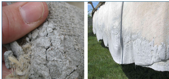
Figure 29. Hardened mortar on drag materials
