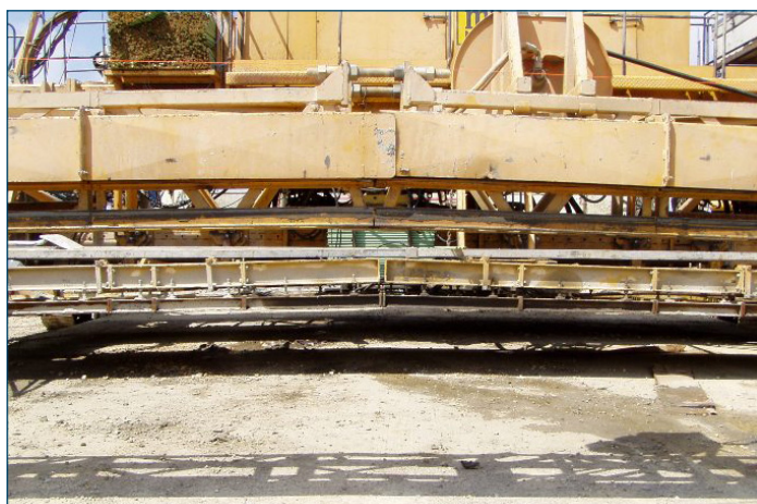
Figure 43. Forming pan set for a crowned pavement
