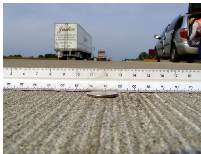
Figure 28. Deep and uniform striations from proper drag texture
