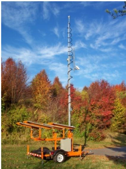
stored in a cabinet on the trailer. The mast folds for transport and telescopes for custom height adjustment. The trailer is equipped with jacks for leveling and stabilization.
