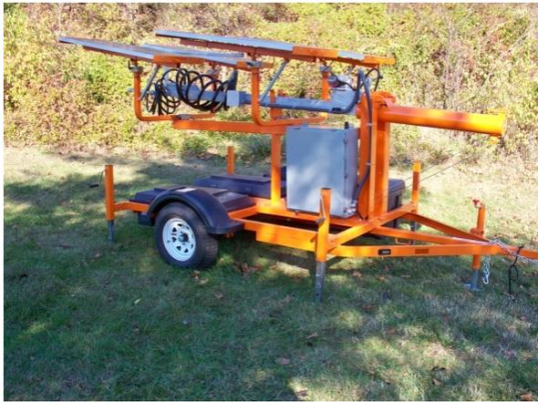
The trailer-mounted portable weather station was received in December 2009. The station is equipped with four moveable solar panels, an electric 30-foot mast, an all-in-one wind, precipitation, air temperature, barometric pressure, and relative humidity sensor unit, a cabled soil/pavement temperature probe, and a non-contact infrared pavement temperature sensor. The sensors are removed for transport and are
