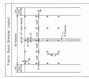
Longitudinal Lap - No more than 12" with the top layer in direction Fabric = 15' wide x 300' long. of paving.
