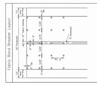
Longitudinal Lap - No more than 12" with the top layer in direction Fabric = 15' wide x 300' long. of paving. STP-S-C091(90)--5E-91
