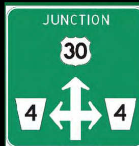
Example of Diagrammatic Signing for At-Grade Expressway Intersection Used in Nebraska
