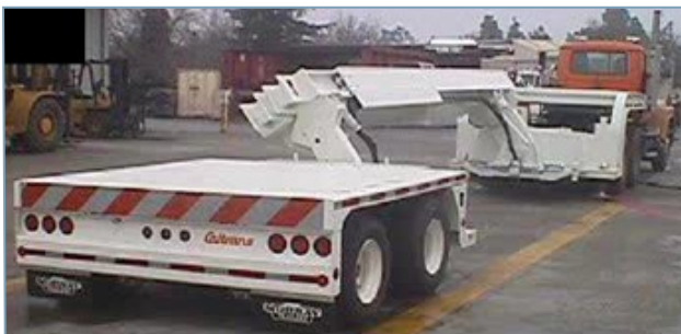
Developed by the California Department of Transportation (Caltrans), the Balsi Beam has great potential for protecting exposed workers in short-duration work operations
