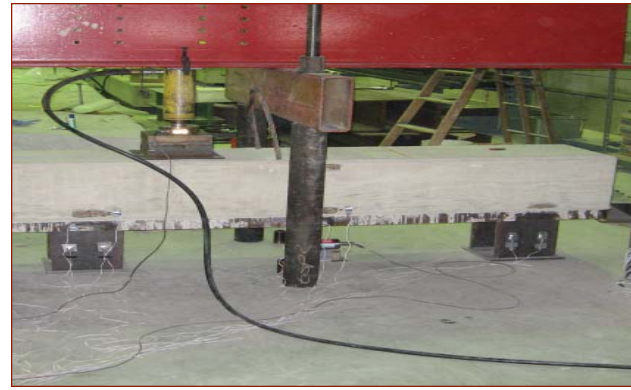
Laboratory testing on a precast abutment cap
