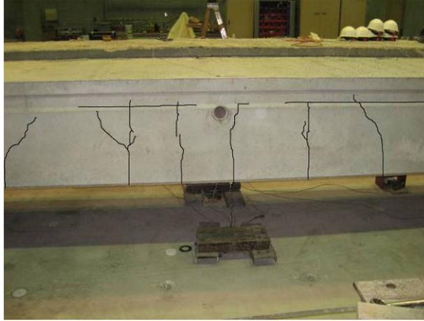
**Figure 4.7. Photograph of flexural cracking after flexure test**
