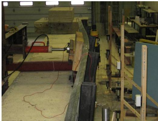
**Figure 4.25. Photograph of deflected guardrail during test 4**
