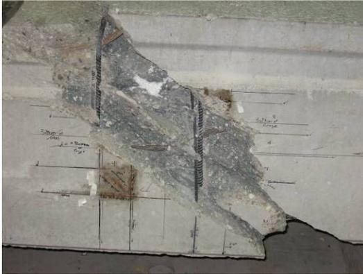
**a. shear crack after failure**
