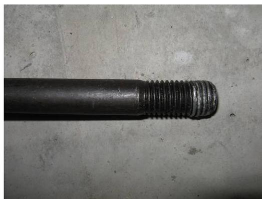
**d. bolt with sheared base plate threads**
