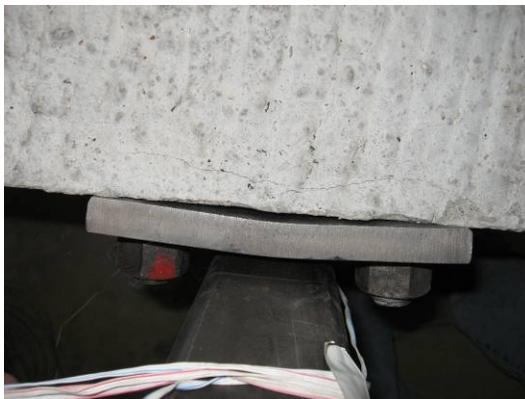
**a. yielded base plate and concrete cracking**
