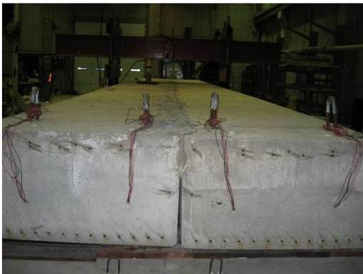
c. girders with the shear key cast.
