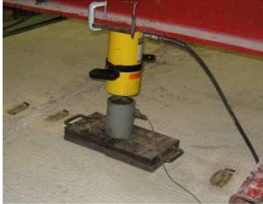
**Figure 3.5. Photograph of tandem wheel footprint used during the variable post-tensioning force tests**
