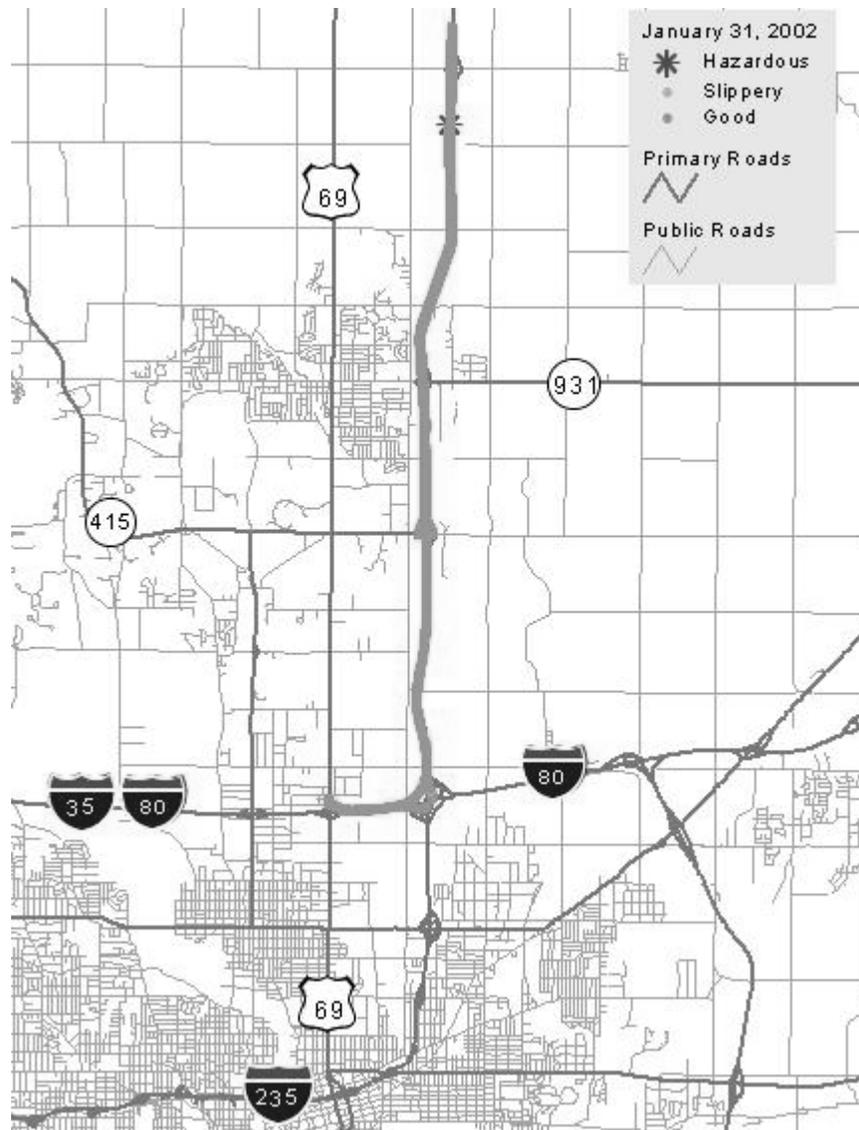
**Figure 15: Sample Friction Measurements taken January 31, 2002**
