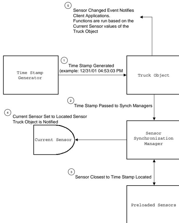
**Figure 37: Sensor Synchronization Process**
