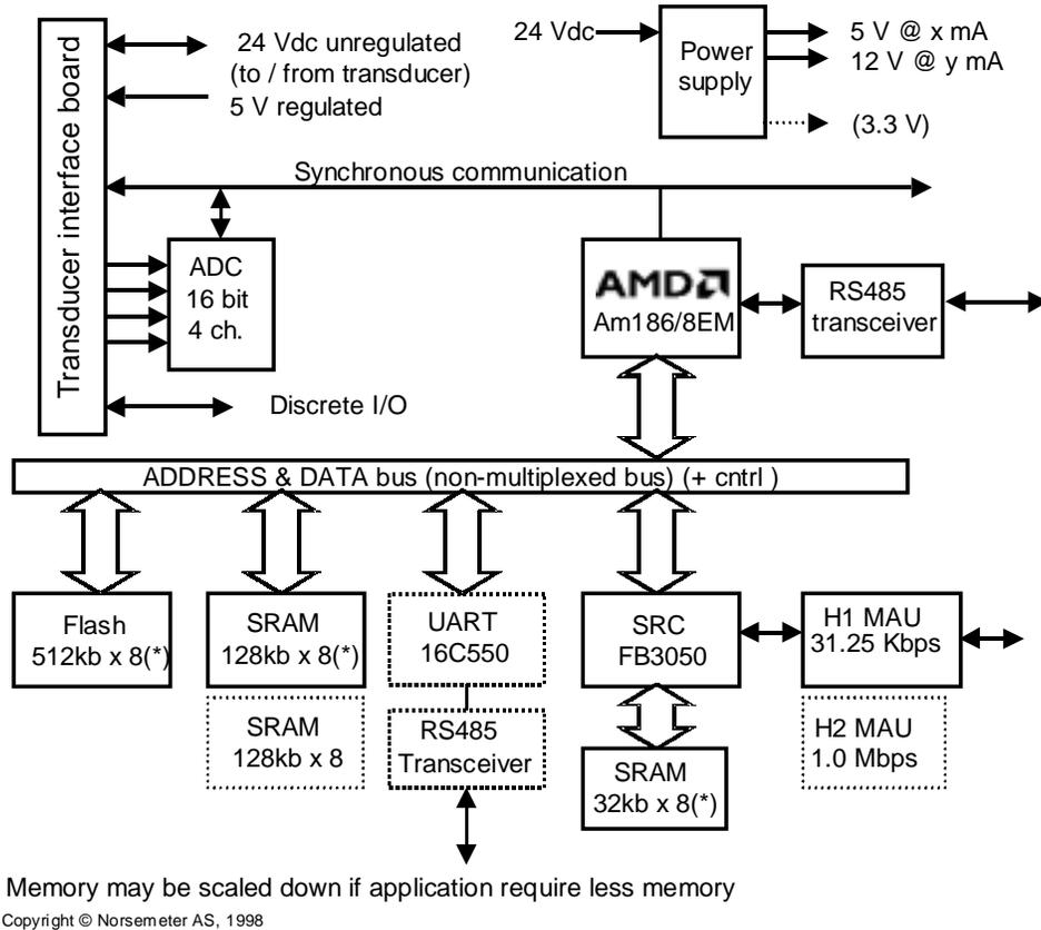
**Figure 11: Schematic of SALTAR Mk I Computer**
