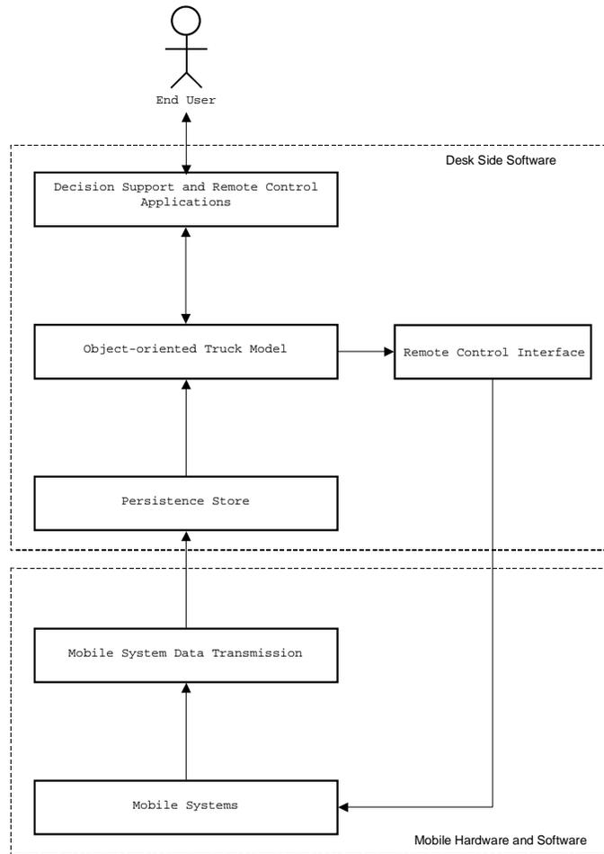
**Figure 34: Software Conceptual Architecture**
