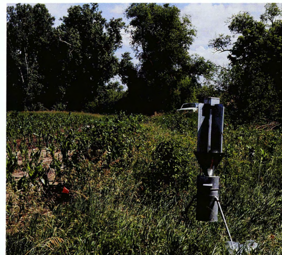
Figure 16. Blacklight trap equipped with 15-watt bulb, photocell, and 12-volt battery.
